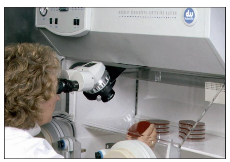
The Don Whitley Scientific stereo zoom microscope is supplied with an 0.5x objective lens, a pair of 10x eyepieces and a trinocular head. The third port permits a camera to be attached by the use of a suitable adapter.
